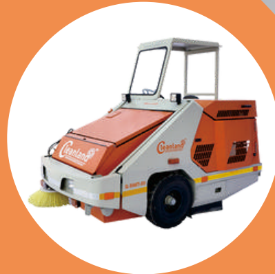
600 Litres | 35 HP Mitsubishi Engine | Imported Hydraulic Pump
