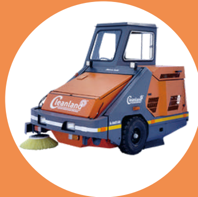
620 Litres | 35 HP Mitsubishi Engine | Imported Hydraulic Pump
